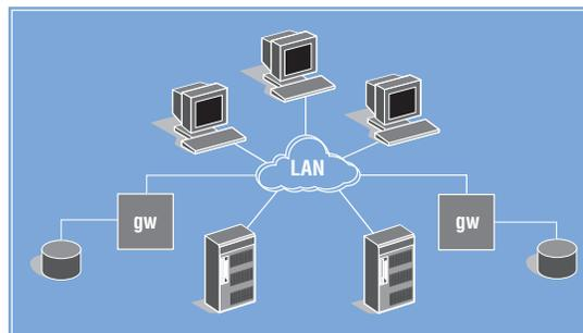
NAS gateway: A NAS device without integrated storage (i.e., just the NAS processor). Instead, the NAS device connects externally to storage by direct attachment or by a SAN.
