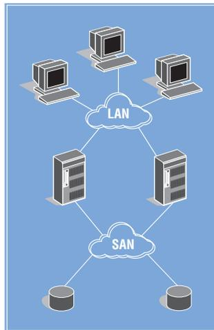
A SAN is a dedicated network for storage devices and the processors that access those devices. SANs today are usually built using Fibre Channel technology, but the concept of a SAN is independent of the underlying type of network.
