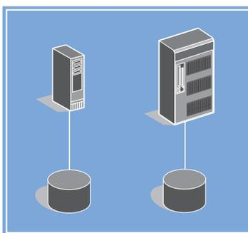
DAS: Direct Attached Storage. Storage (usually disk or tape) is directly attached by a cable to the computer processor. (The hard disk drive inside a PC or a tape drive attached to a single server are simple types of DAS.) I/O requests (also called protocols or commands) access devices directly.
