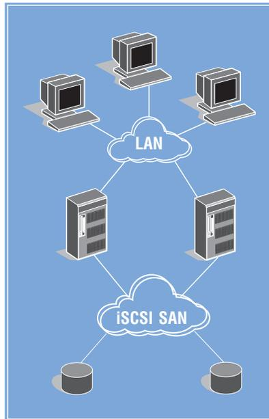
iSCSI is a proposed industry-standard that allows SCSI I/O commands to be sent over a network using the popular TCP/IP protocol. This is analogous to the way SCSI commands are already mapped to Fibre Channel, parallel SCSI, and SSA media. The proposal was made to the IETF (Internet Engineering Task Force) standards body jointly by Cisco Systems, Inc. and IBM.
