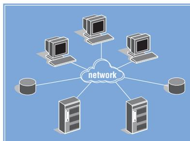
Network attach—one or more processors are connected to one or more storage devices.
