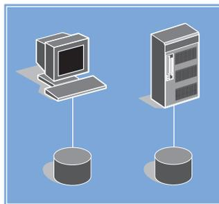
Direct attach—a single storage device is connected to a single processor (host).
